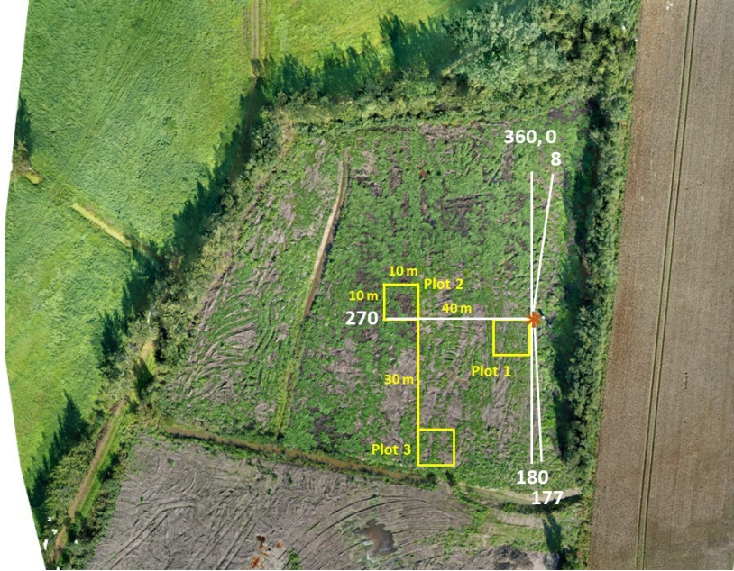
Figure 1: Measurement site captured by drone on 1 September 2020. The location of the eddy covariance tower (red asterisk), the cardinal directions (white), approved wind directions for EC data (white), and the three sample plots (yellow), each 100 m 2 in size, are illustrated in the figure.
